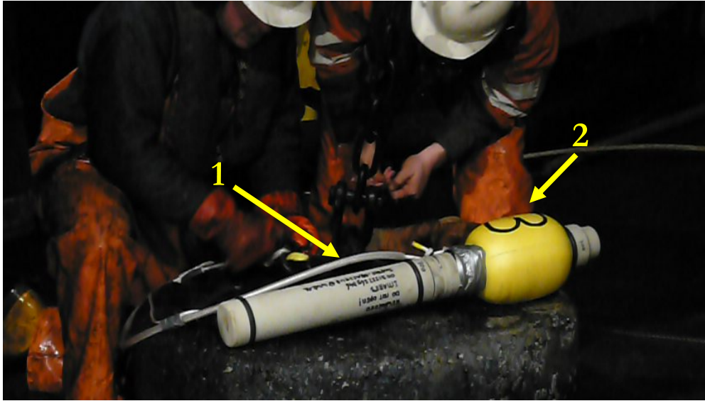
Figure 5. The new T-POD attachment. Kevlar cable with rubber tubing (1) and buoy (2) for additional buoyancy.
