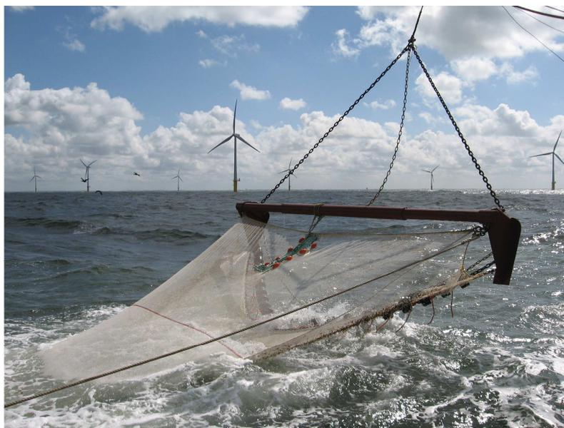
Figure 3.1: One of the 6 m beam trawls used for sampling the demersal fish community. Attached is the 20 mm net. In the middle of the net the CTD device is visible. (photo: R. ter Hofstede).
